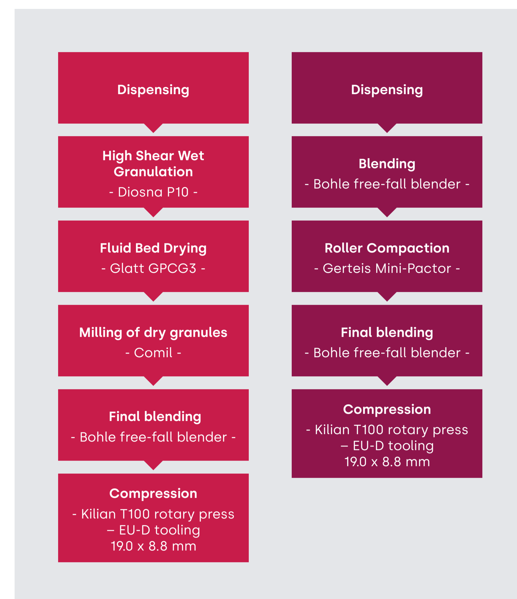
Figure 3: Process train and equipment for wet granulation (first column) and dry granulation process (second column)
